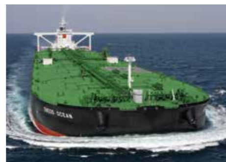
原油タンカー Deadweight capacity: 312,181 tons, 機関出力: 23,620kW Crude oil tanker Deadweight capacity: 312,181 tons, engine power: 23,620kW
