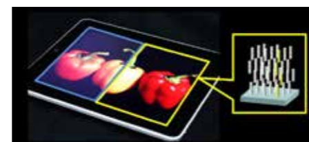
IPS-LCDの視野角拡大 (左:NVフィルムなし、右:NVフィルムあり、吹出し:液晶分子の配向) Improvement of Viewing Angle of IPS-LCDs (Left: without NV, Right: with NV and Alignment of Liquid Crystalline Polymers)
